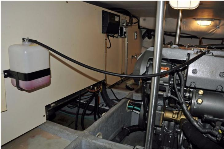
**Coolant recovery bottle plumbing should be routed so that it is not in harm's way, and so that it does not impede access around the engine. Most recovery bottles are plumbed from the bottom, however, some, like the one shown here use an internal pick up tube.**
