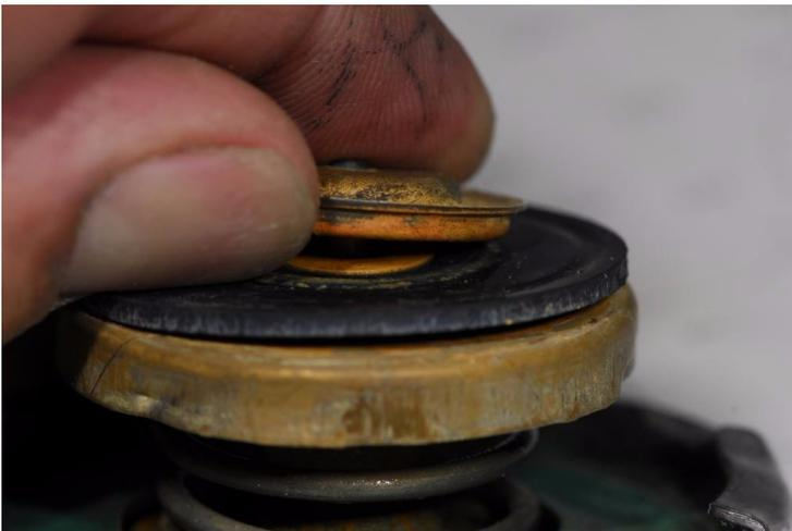
**Pressure caps are comprised of several parts, including gaskets, springs and a check valve, all of which must be in good working order for the coolant recovery bottle system to work properly.**
