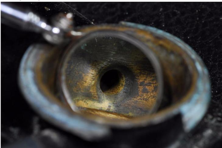
**The port located in the expansion tank fill neck allows coolant to flow to the recovery bottle when the cap reaches its rated pressure. When the system cools and contracts, a vacuum is formed, drawing coolant back through this port and into the expansion tank. In order for this to work, the cap's upper gasket must form an airtight seal, and thus it must be rubber or a soft gasket material.**
