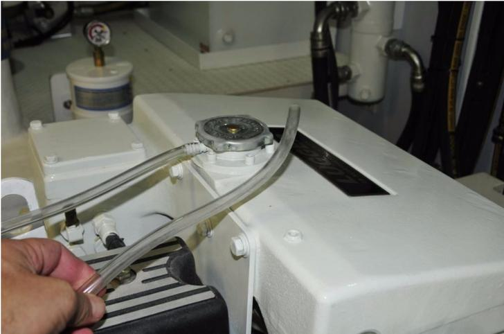
**While it's all too commonly used, clear PVC hose is not robust enough for coolant applications, it collapses, chafes and melts far too easily. Type B fuel hose makes for a far better choice.**
