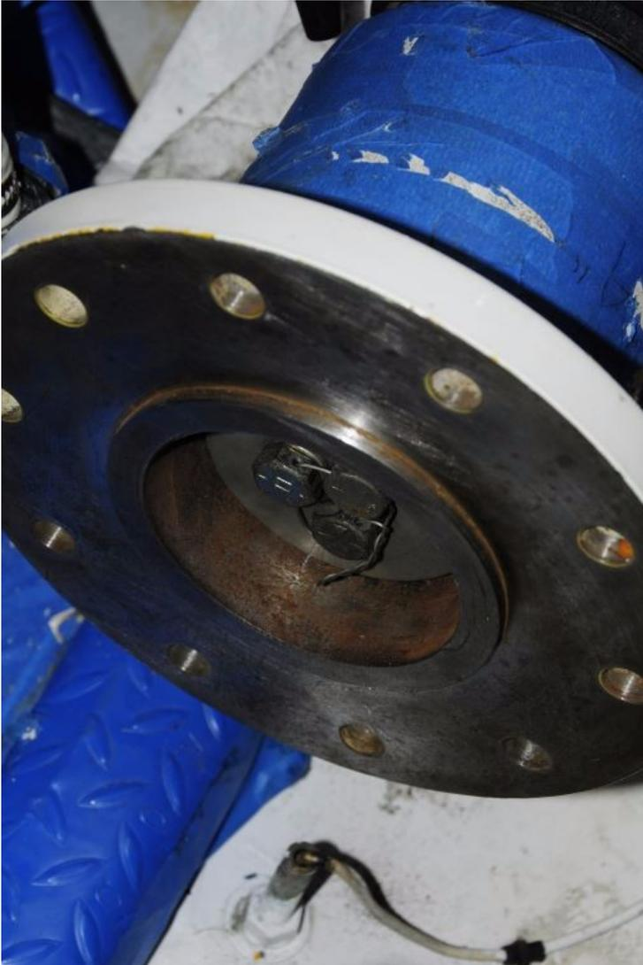
**The pilot bushing, the protruding ring within the coupling face, shown here, ensures that the two couplings are centered on each other. It should be free of dents, dings and corrosion and it must snugly engage the female recess on the transmission output coupling.**
