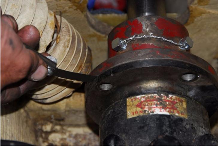
**Tried and true, using feeler gauges to measure and close the gap between propeller shaft and transmission output couplings.**
