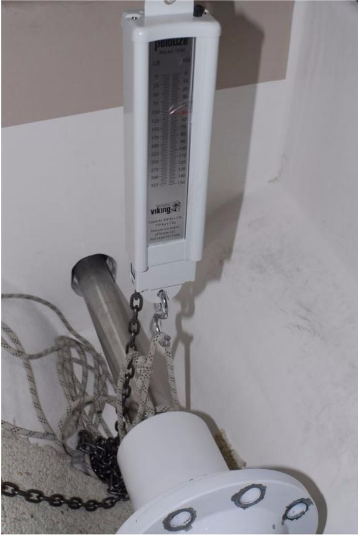
**Eliminating shaft droop can be accomplished using a hanging or conventional scale, thereby accounting for the weight of the shaft and coupling.**
