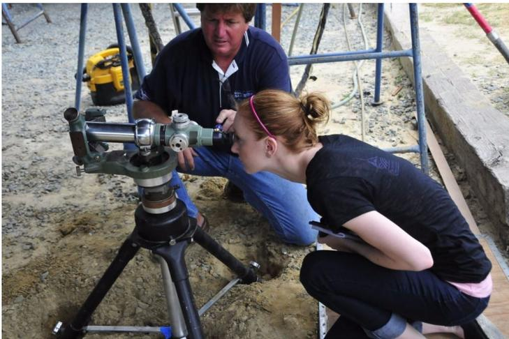
**Optically 'sighting through' to, among other things, avoid aligning the transmission output coupling to a sagging or drooping shaft, is a critical aspect of the alignment process.**
