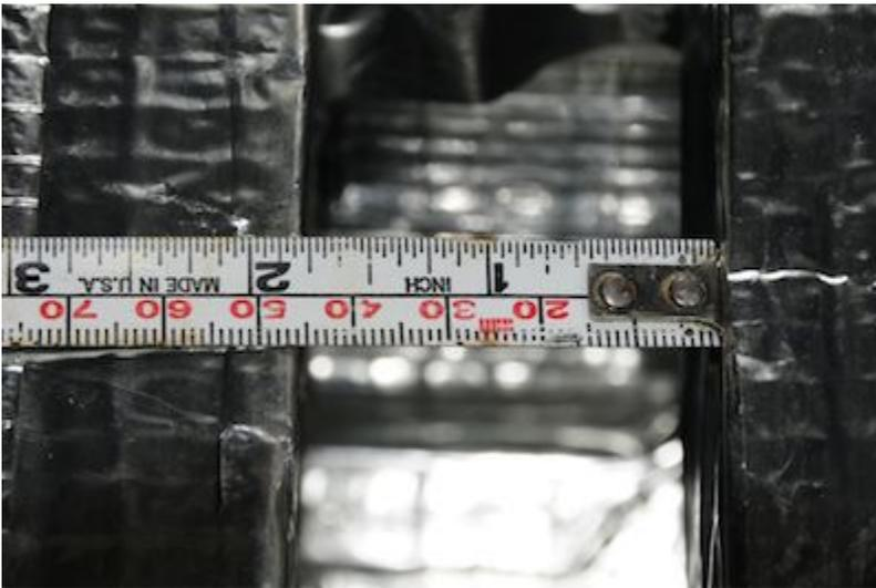
Air inlet openings must be measured at their narrowest restriction, often what begins large on deck, is constricted by the time it enters the engine room.
