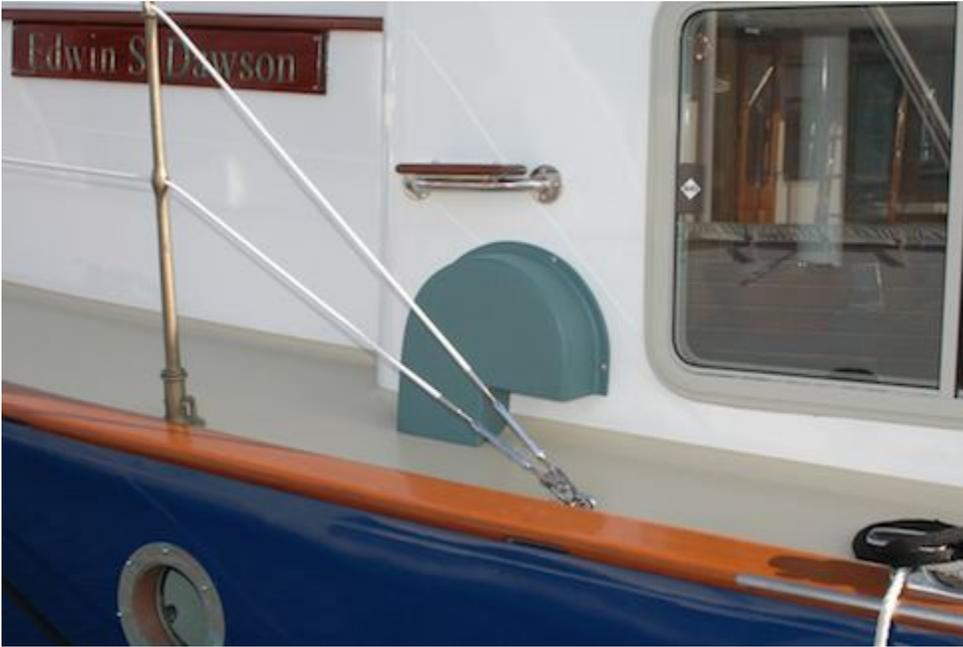
This engine intake includes a 180° gooseneck that is designed to prevent ingestion of water. Consideration should be given to engine air intake locations: those that are subject to heavy spray are less than ideal, and if chosen should include a means of water exclusion or separation.
