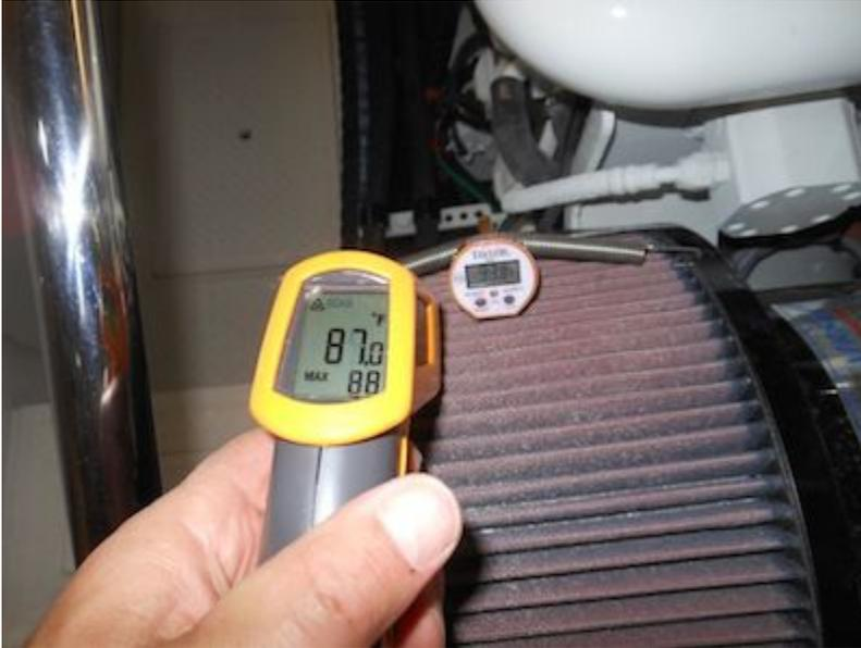
**For the sake of consistency, and to comply with engine manufacturer guidelines, engine room air temperature should be measured at the engine inlet or filter. Digital probe type thermometers should be used; avoid infrared pyrometers for this measurement as they often yield inaccurate readings.**
