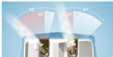
The single units of the Zeus® Pod Drive System can be steered independently. The amount of each pod's thrust can be varied as required, thanks to a special mechanism which is electronically controlled. This means much smoother and accurate maneuverability.
