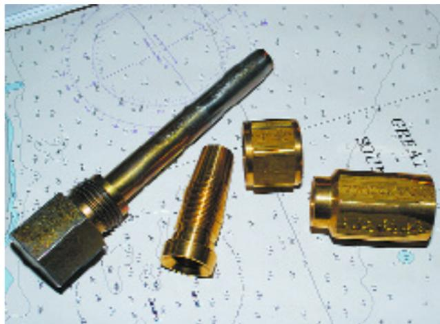
A Parker field-assembled hose connector and the mandrel tool that's used to assemble it. These fittings are extremely durable and reliable and lend themselves to use in boat construction, repair, modification, and service work.
