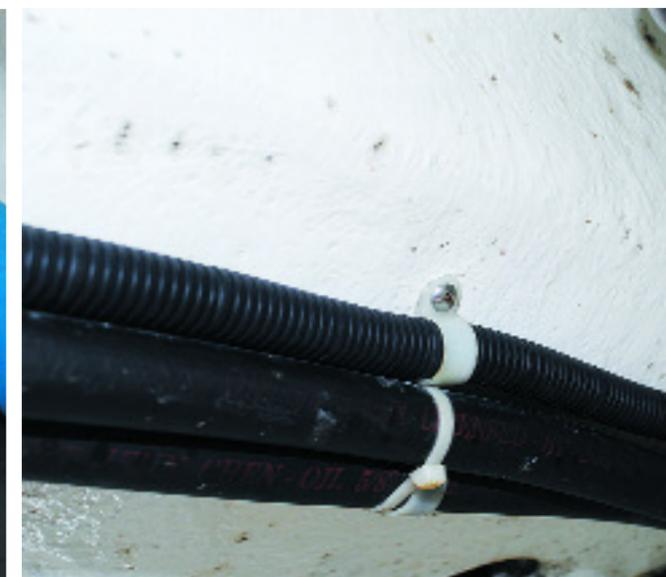
Opposite page: In order to comply with ABYC guidelines, all metallic fuel system components, such as this stainless steel distribution priming manifold, must be connected to the vessel's bonding system. Above left and right: Securing fuel lines by using plastic wire ties is acceptable; however, it should be the exception rather than the rule, and plastic wire ties should never be used in locations where fuel lines pass over machinery with moving parts, such as engines and generators.
