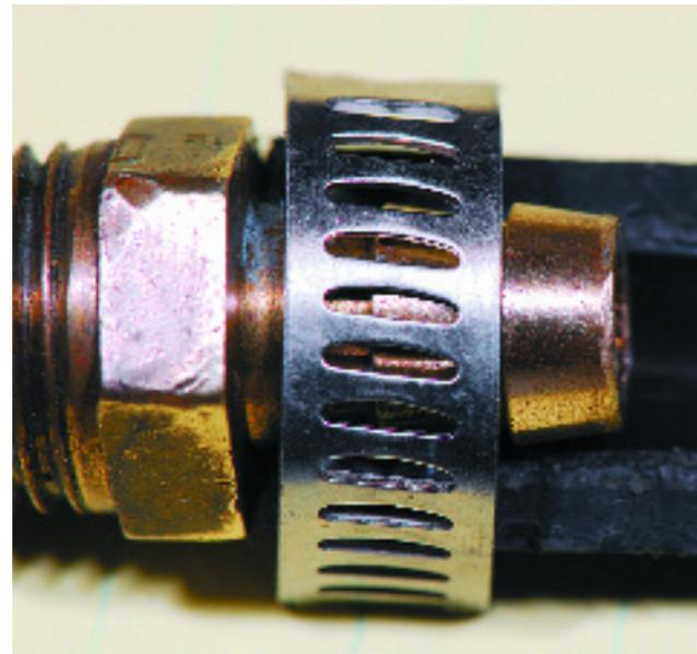
A cutaway view of a hose and barb assembly. It's important to note that the length of this barb prohibits the installation of double clamps.
