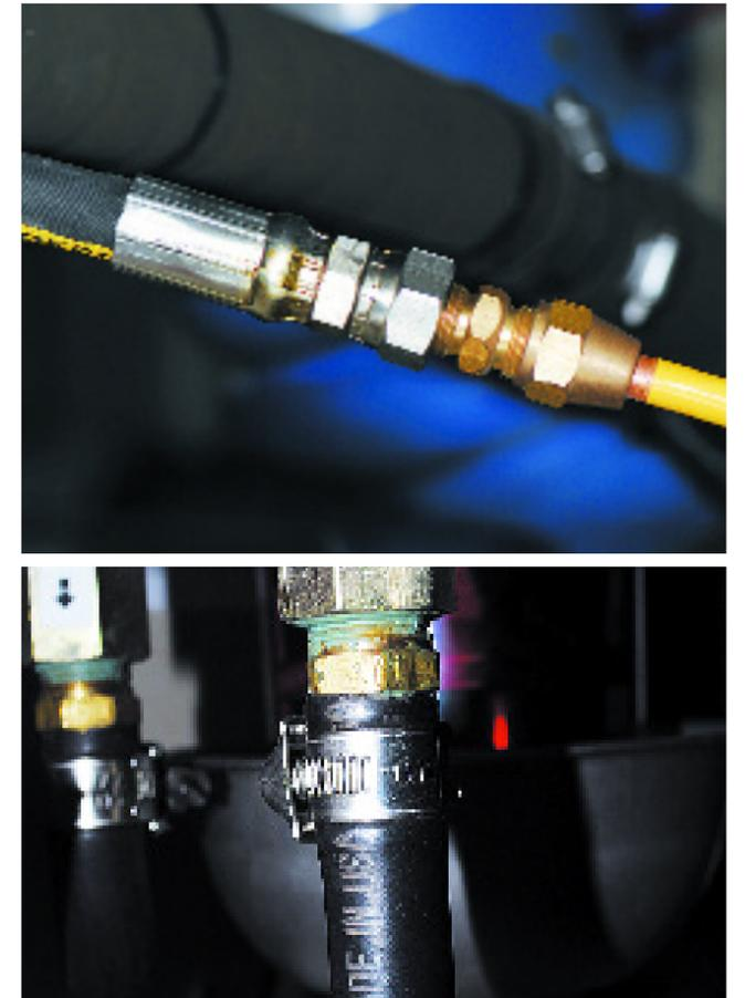
Top: Where the transition is made between rigid metallic pipe and hose (at the attachment point to the engine, for instance), the pipe must be completely immobilized to prevent movement- or vibration-induced fractures. Above: The most common method of terminating ordinary fuel hose is using a high-quality clamp and barb. This barb will fully accommodate only a single clamp, which is entirely acceptable provided it's all stainless steel and the band is not perforated.
