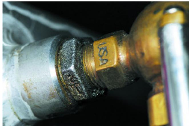
Left: Swaged fittings, such as the one shown on the right, are an alternative to field-attachable hose ends. They are not reusable in that they cannot be detached from the hose once compressed. An advantage is that they are available in stainless steel. Right: Threaded NPT pipe connections are among the least reliable where fuel systems are concerned. Threads should be sealed with a suitable liquid or paste compound such as Loctite 567, 515, or 518.
