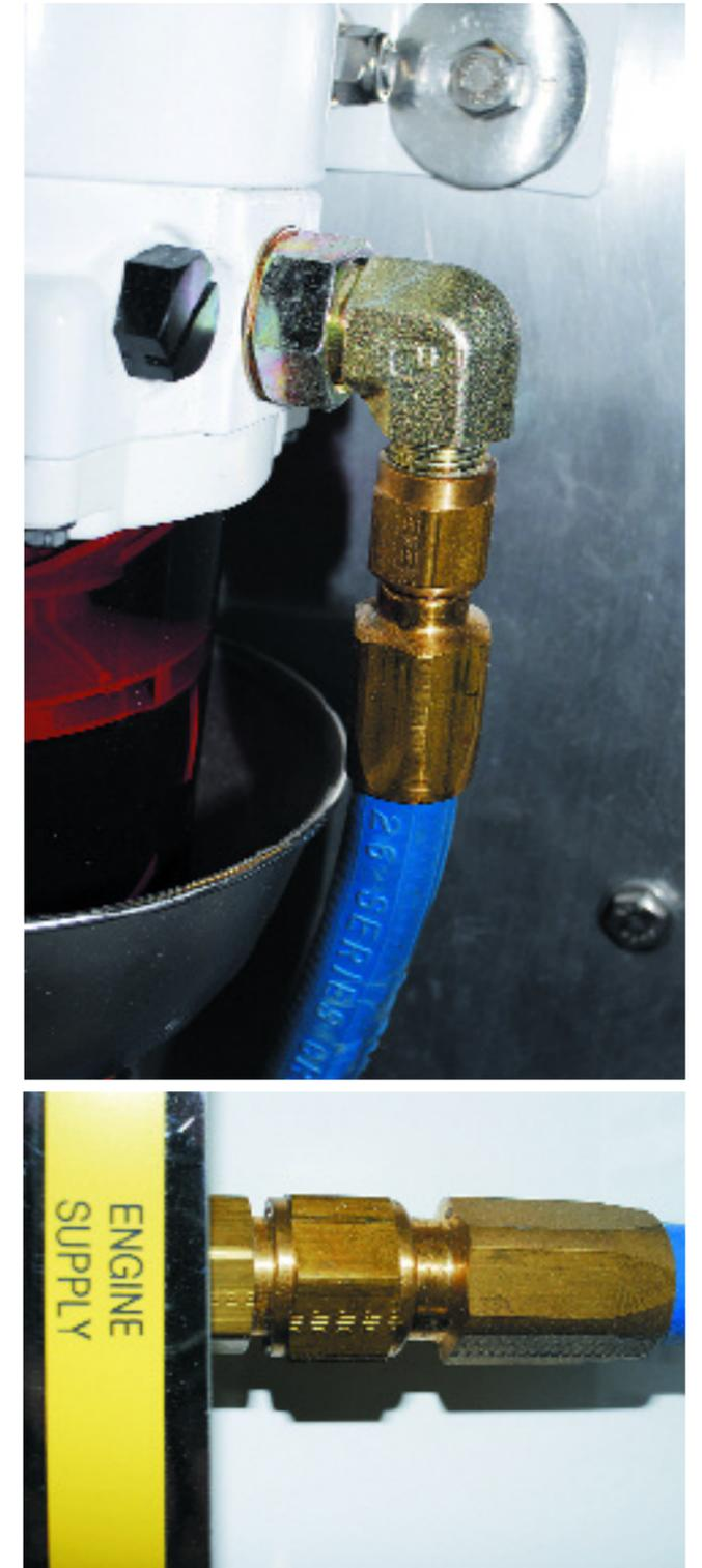
Top: All Parker/Racor fittings used on Turbine series filters are of the JIC variety, which means they have a flare angle of 37 degrees. Here, a cadmium-plated 90-degree fitting is connected to a brass field-attachable hose end. This makes for a virtually leakproof seal. Above: An assembled and installed field-attachable hose end. Notice the "JIC" nomenclature.
